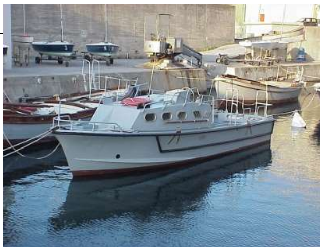
B. Length: 8.5 m, Width: 2.3 m • Material: fiberglass and iron
